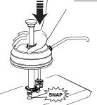
Pump is fully engaged when top surface of pouch fitment touches pump connector rim.
